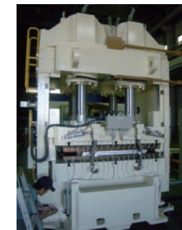
1,000 ton press for insulation sheet manufacture
